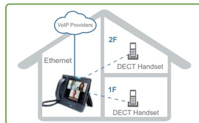
Multi-user VoIP calling with cordless HD DECT CATiq2.0 handsets connected to IP3092D model Communicator
